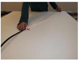
The tail may be placed anywhere on your panel, ideally the ferrule should point towards the light source and not be less than 50mm from the edge. Ensure that the tail will reach to the around 50mm beyond the furthest edge of the panel.
